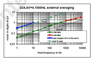
Figure 18: Output voltage noise over sampling rate
