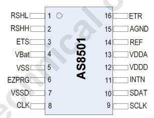
Figure 2: Schematic Package outline SOIC 16
