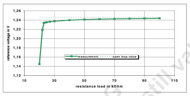
Figure 4: Reference voltage as function of resistance load
