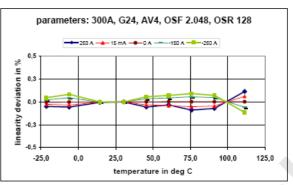
Figure 14: Linearity deviation for different currents over temperature
