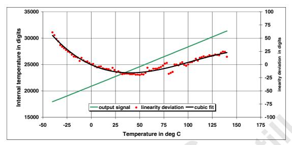
Figure 7: Measurement of internal temperature sensor over oil bath temperature
