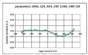
Figure 15: Linearity deviation over input signal
