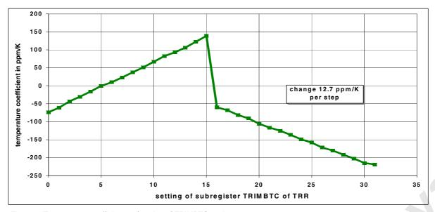
Figure 6: Temperature coefficient as function of TRIMBTC setting
