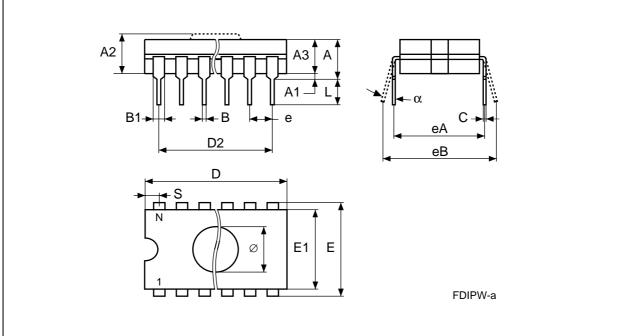
Table 14. PDIP40 - 40 pin Plastic DIP, 600 mils width, Package Mechanical Data
