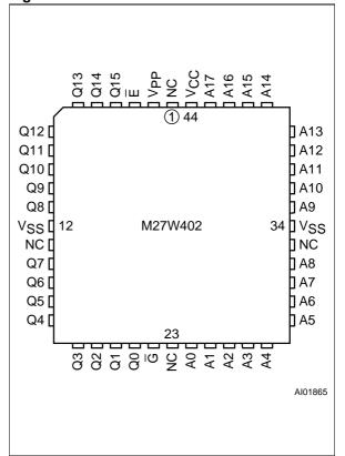
Figure 2C. TSOP Connections
