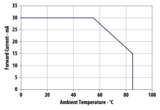
**Maximum Forward Current vs Ambient Temperature**
